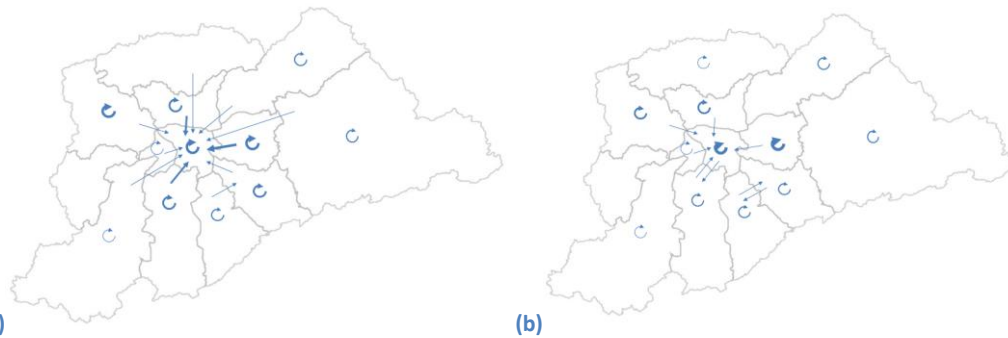
Figure 18: Trips at morning peak in 2012 (5:00 a.m. to 8:00 a.m.) – 80% of the most significant routes. (a) Mass transportation. (b) Private transport. The thickness of each arrow is proportional to the density of flow.
